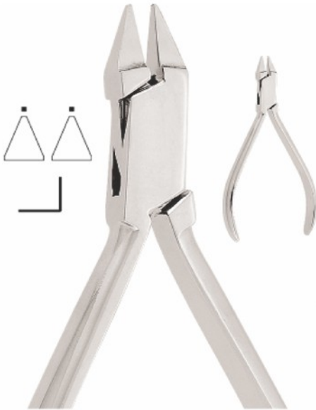
F15-071 Adams Plier Adams pliers for bending wire arches and bends right angles for wires up to .022", .025 tip to beak. Length 13cm
